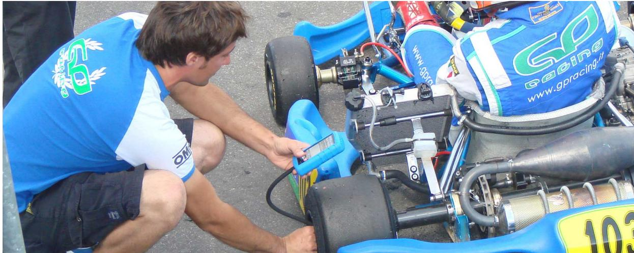
A tire pressure gauge is a popular basic tool to have at the kart track. While most are not as fancy as the electronic unit pictured here, a pressure gauge is a must-have for karting. (PC: Prisma Electronics)
