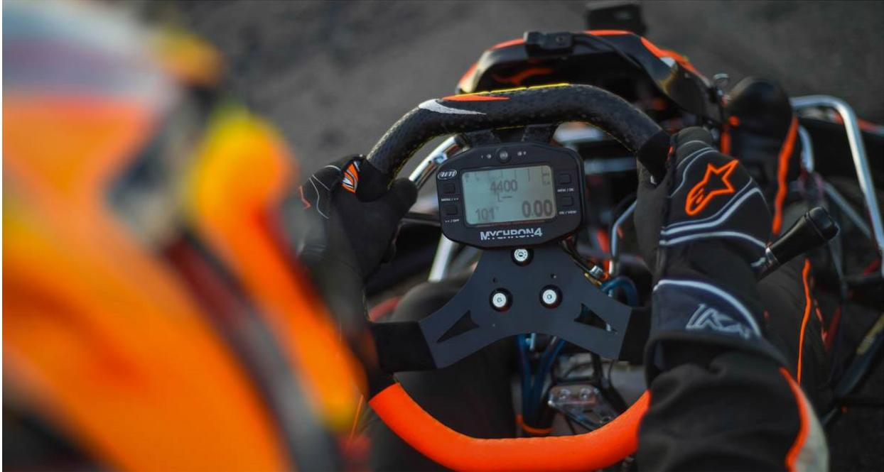
A data acquisition system like this one, pictured attached to a driver's steering wheel, is highly useful for many reasons. Depending on the functions the system has, a driver and kart's lap time, RPM, engine temperature, and even GPS position on the track can be found within the data these systems store or display in real time.
