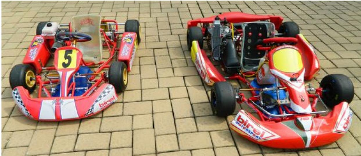
Drivers of different ages can enter into karting through the class system, which allows for a progressive increase in the size of the kart, and resultant performance. Here, a kid kart (left) sits alongside a cadet kart powered by a Rotax MicroMax engine. (PC: Radne)
