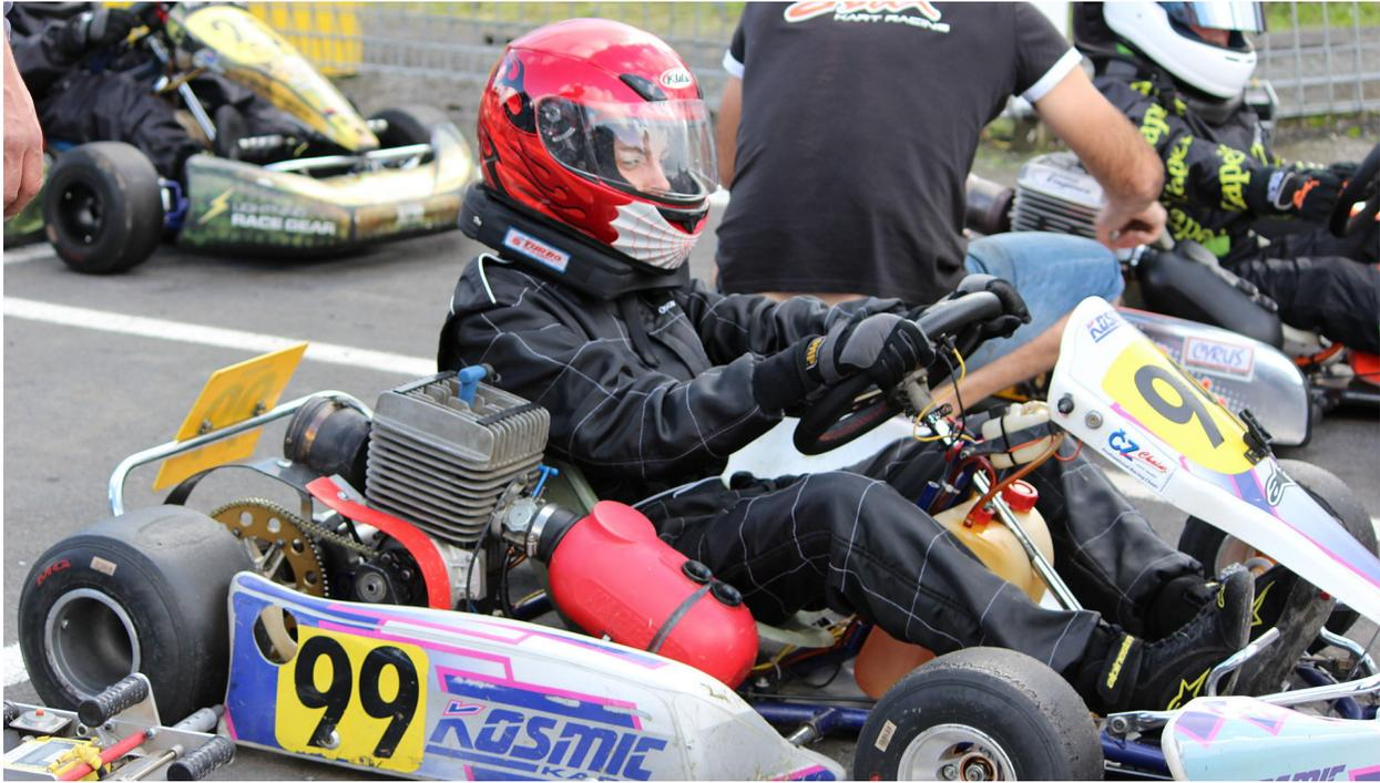
A legacy of karting's earlier development, the 100cc engine displacement category has been mostly usurped by 125cc engines. However, exceptions still exist in karting. Initially implemented in the early 1980s, the 100cc Yamaha KT100 engine package is famed for its durability and close racing action. Of all 100cc engines, this package is the most common still in use today. (PC: Oscar King)
