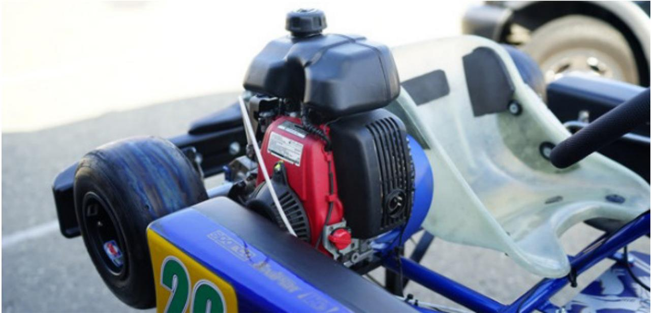
In recent years, the Honda Gxh50 engine has been the go-to engine package for most Kid Kart classes across the country. 50cc engines produce between 2 and 4 horsepower, and will propel a Kid Kart to a top speed of roughly 40 mph. (PC: Ekartingnews.com)
