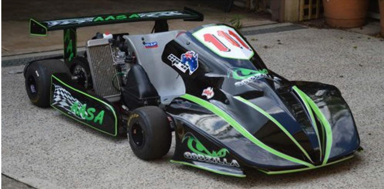
Another slight variation on road racing and endurance karts are so called 'super karts.' With large engines, tires, and often additional aerodynamic bodywork, these karts are capable of speeds at times in excess of 150 miles per hour. While not as common a sight at the track, they are hard to miss when they are there, as their pace through the corners and down the straightaways is dramatic. (PC: KartPulse)
