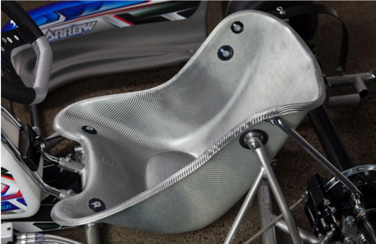
The kart seat has evolved over the years considerably. Note the flat bottom of this seat, which allows for a lower mounting position. The silver-sheen of this karting seat suggests that this seat features reinforced cross-weaving of the fiberglass, which adds durability and performance. Also, note the silver seat strut mounted to the rear of the seat, providing additional grip to the rear tires. (PC: KartSport NZ)
