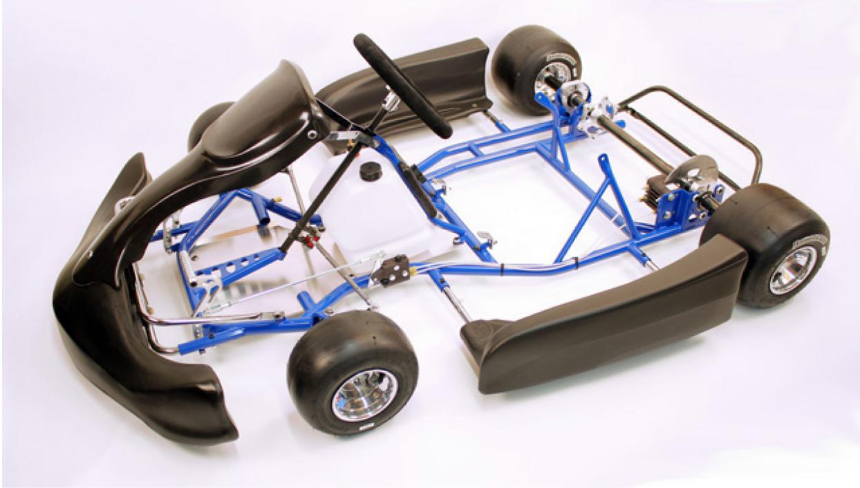
A kart chassis (in blue) with associated componentry, with the seat absent. In this case, this chassis is intended for sprint kart competition. Note the steering, solid rear axle, brake location, central gas tank, and plastic bodywork. The two parallel rails on the right of the chassis are the typical location for mounting an engine. (PC: Comet Kart Sales)
