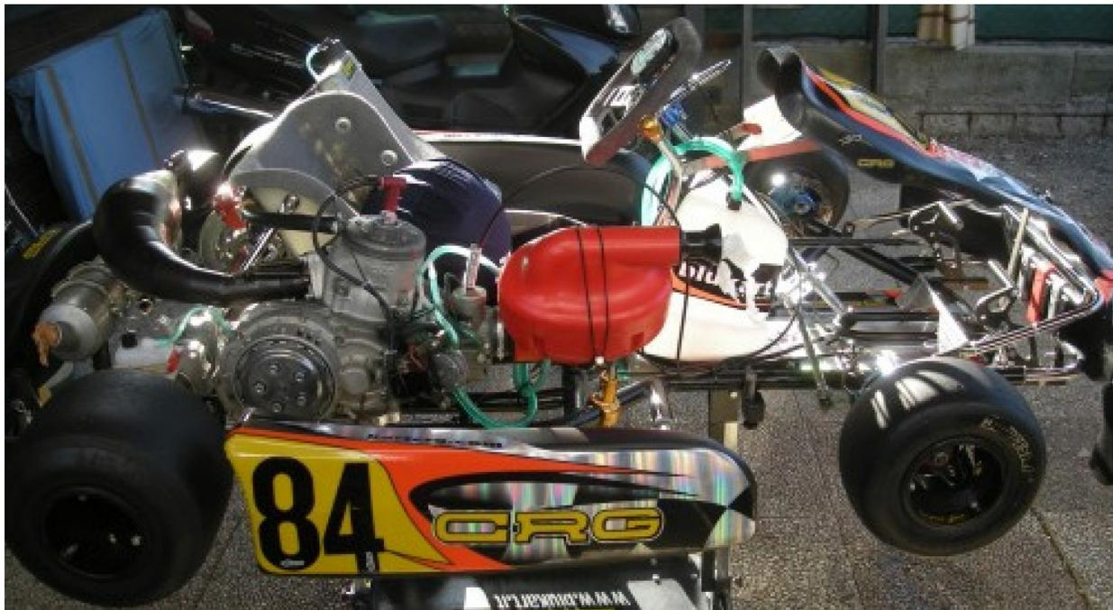
While exciting to watch, a shifter kart engine is typically the most complex and temperamental of all engine package types in karting. In their most extreme form, the ICC shifter engine (pictured), driving one becomes as much about hanging on as it does about being smooth and relaxed. (PC: Solokart)
