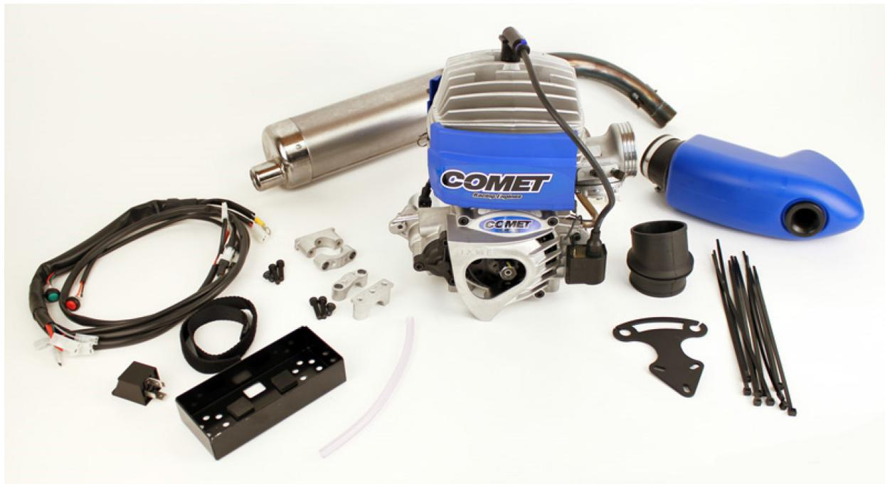
In recent years, ‘Touch and Go’ type engine technology has migrated from higher-power classes to the 60-80cc engine. Examples of these include the Parilla Mini-Swift (pictured) and the Rotax Micro Max. Here, a Mini-Swift engine package is shown in disassembled form. From left to right: Battery box and wiring loom, exhaust (background), engine, air intake and filter. (PC: Comet Kart Sales)
