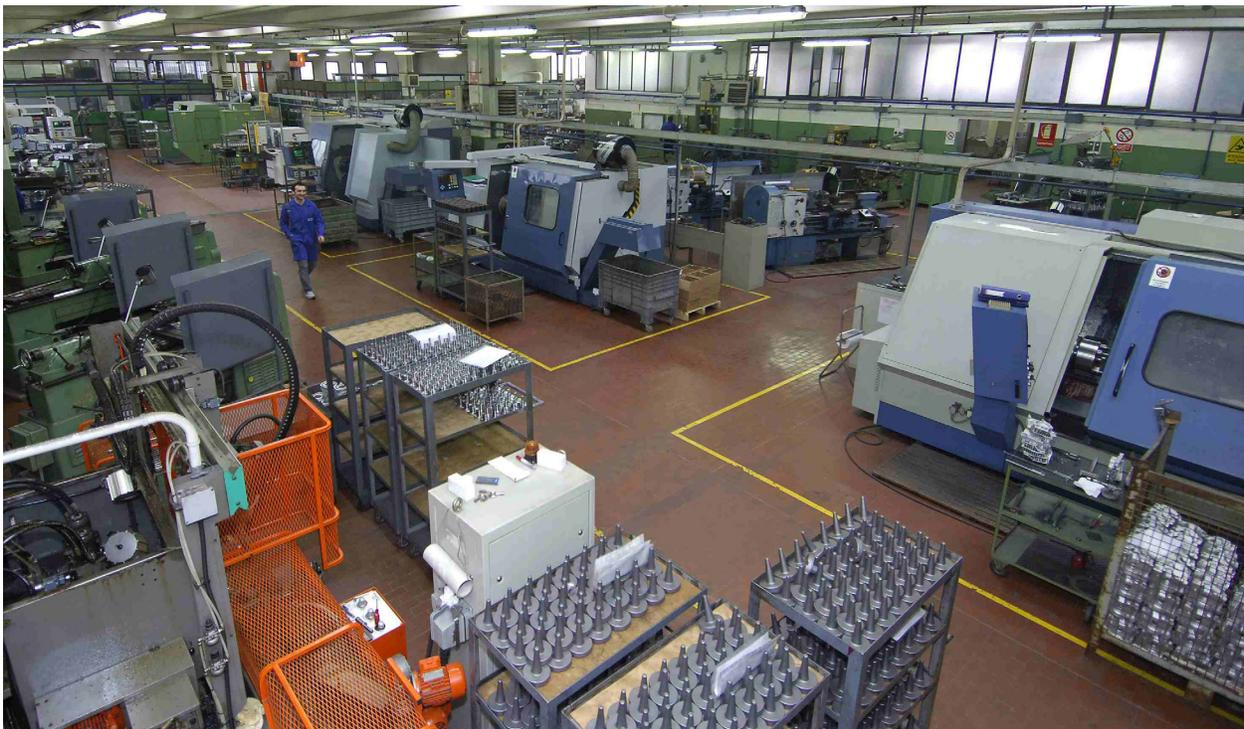
Kart engines of today are produced using advanced materials, manufacturing techniques, and computer-aided design to ensure that the greatest level of parity between each engine is achieved. In this photo, the CNC machines and manufacturing floor of an IAME Karting Engine factory is shown. (PC: IAME Karting)
