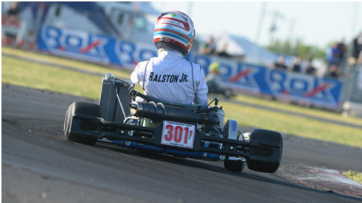
Every modern racing go kart is the result of decades of development by major kart manufacturers. The engineered ability of a kart to ‘hike’ its inside rear tire in a corner is the key to the astounding cornering ability most karts produce. Here, a kart demonstrates perfect wheel hike as it travels around a corner. (PC: OnTrack Promotions)
