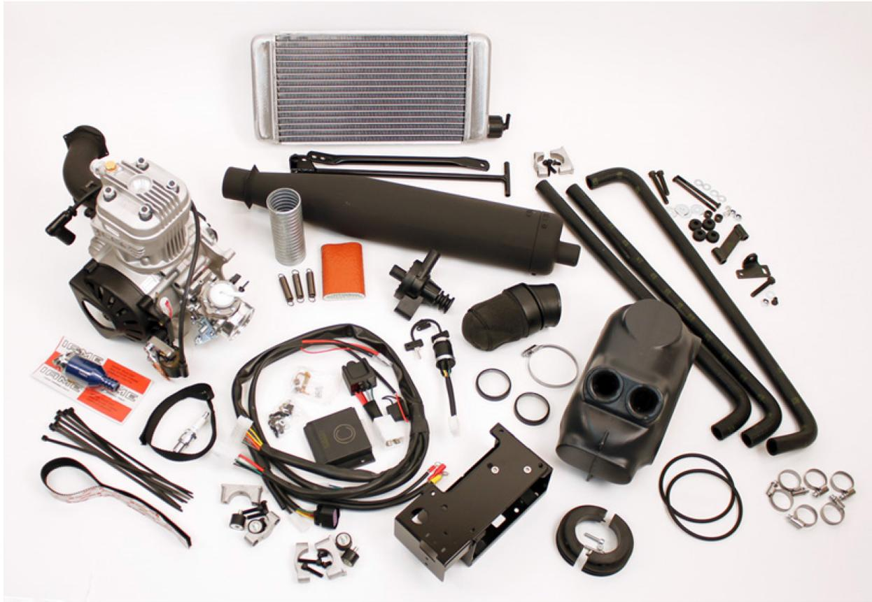
125cc engines come in many forms. However, as you can see from this photo, most 125cc engine packages are significantly more complex than their smaller displacement siblings. Pictured is the componentry of a 125cc IAME X30 engine, one of the go-to Touch and Go (TaG) engine packages on the market and in use today. Note the larger exhaust, radiator (at top of picture), radiator hoses, wiring loom, battery box, and large air intake and filter. (PC: Comet Kart Sales)
