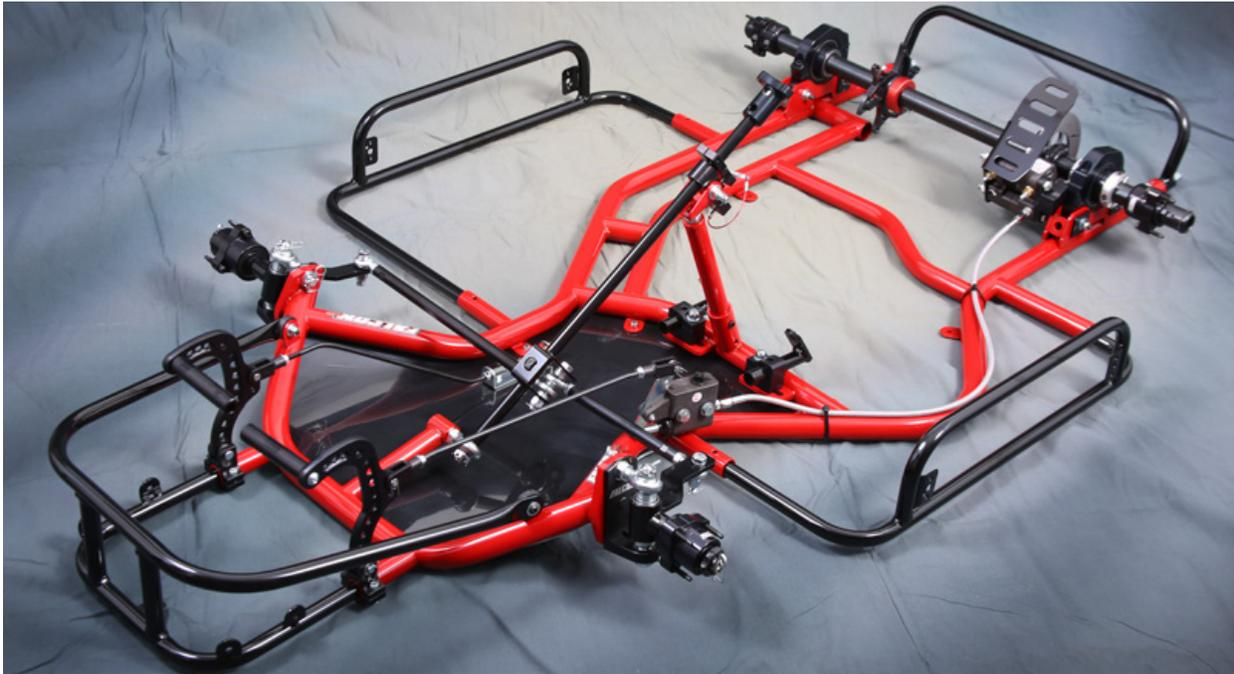
An oval track kart chassis, with seat, tires, and bodywork removed. Note the offset chassis structure (naturally to the left). In many ways, this chassis is exactly the same as a sprint kart chassis, but critical components like the driver's seat position, steering, and even bodywork are offset to cater to left turns.(PC: Southern Express Karting)
