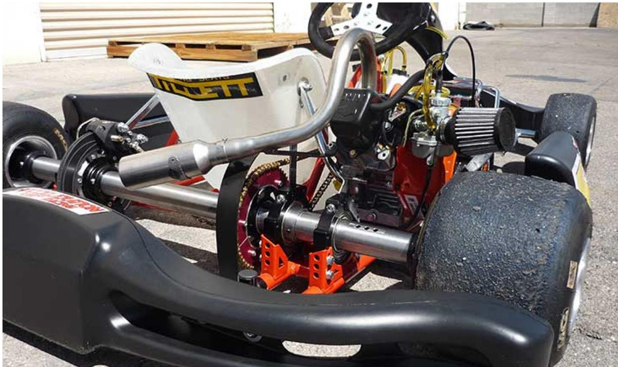
The 4-cycle karting engine has been in use in oval kart racing for decades. It is only recently, however, that the 4-cycle engine has been widely used in sprint kart racing. Note the drive train location, large size of the engine, and split rear sprocket. (PC: Acceleration Karting)
